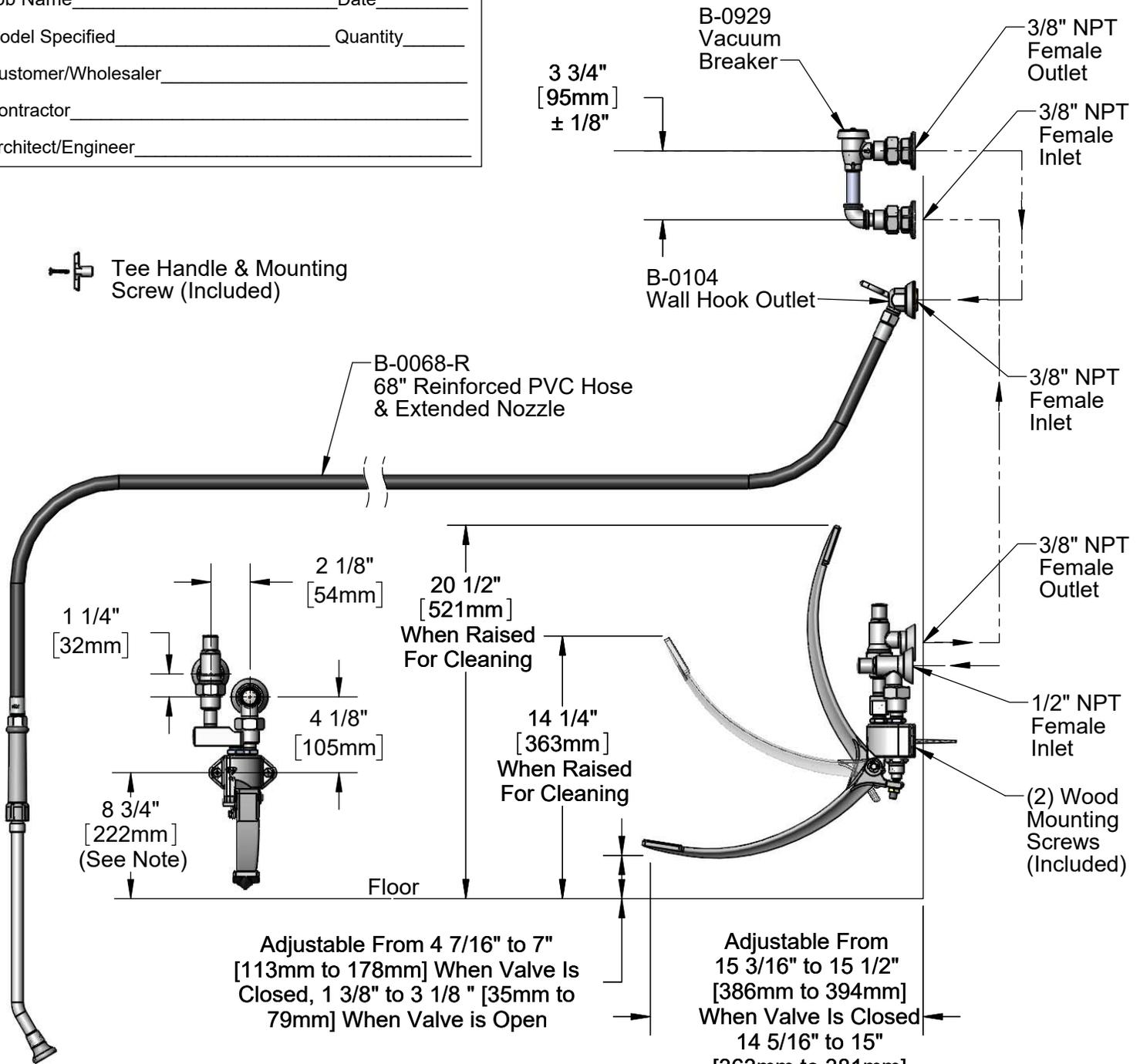
Note: All Pedal Position Dimensions are Based on Minimum Recommended Mounting Height of 8 3/4" [222mm] Above Finished Floors.
