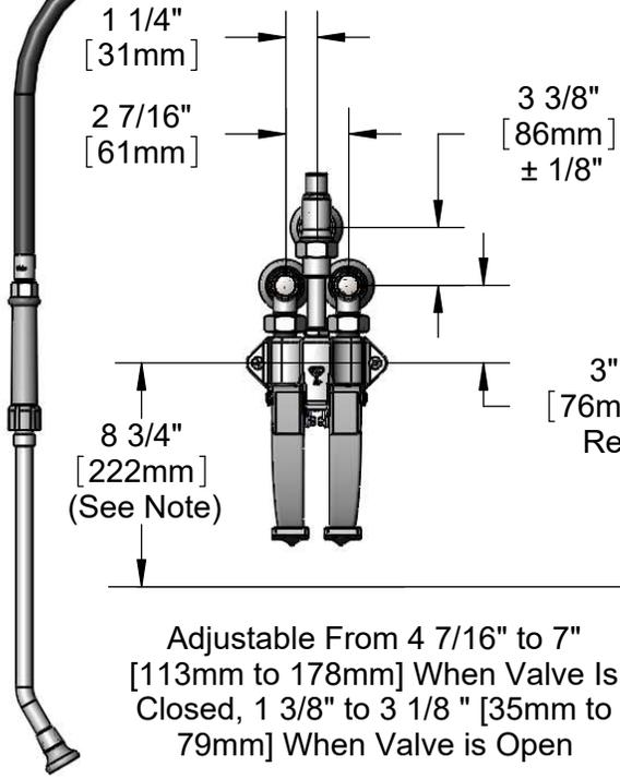
Note: All Pedal Position Dimensions are Based on Minimum Recommended Mounting Height of 8 3/4" [222mm] Above Finished Floors.
