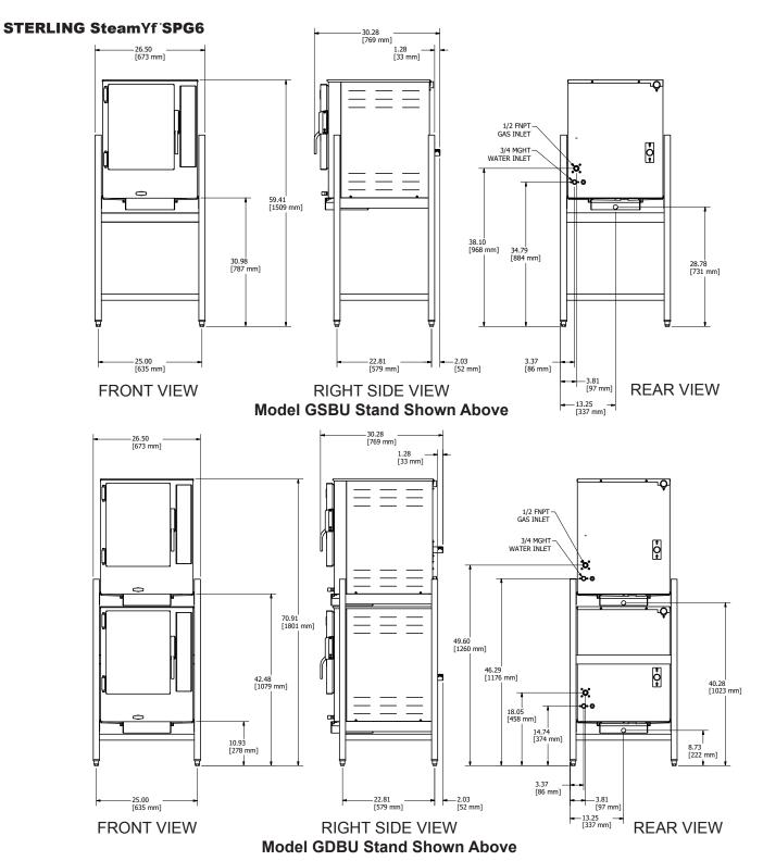
Note: Dimensions do not change for variations in Model Numbers. Bullet Feet and Flanged feet have a 1" adjustment.
