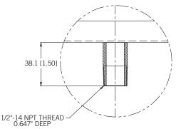
DETAIL "A" DRAIN FULL SCALE
