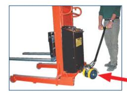
5th Wheel Steering Option for easier mobility and precision steering in confined areas Available only on 1,500 and 2,000 lb models. 8" locking polyurethane wheels. Spring loaded handle. Can be field installed.
