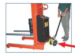
5th Wheel Steering Option for easier mobility and precision steering in confined areas Available only on 1,500 and 2,000 lb models. 8" locking polyurethane wheels. Spring loaded handle. Can be field installed. Order as separate option under Part # 261099
