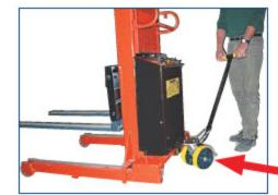
5th Wheel Steering Option for easier mobility and precision steering in confined areas Available only on 1,500 and 2,000 lb models. 8" locking polyurethane wheels. Spring loaded handle. Can be field installed.
