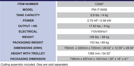
Floor Model Pasta Machine with 8.8-lb Capacity and 3/4 HP
