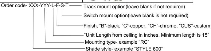
Examples-" 600-SMT-C-24" = Style 600 shade, rigid ceiling mount 3/8" diameter down tube, copper finish, 24" long "800-LGT-CUS-38-S-T" = Style 800 shade, rigid ceiling mount 1 ½" diameter down tube, custom finish, 38" long, switch option, track mount.
