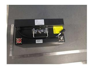
8-LFP-60-EV-NOB Type: Rate Voltage: 25.6V
