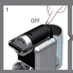
Press and hold Ristretto and Espresso buttons while turning on the machine.
