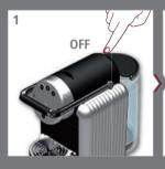
Press and hold Hot water button while turning on the machine.
