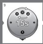
To select New filter, press Ristretto during blinking cycle.
