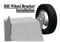
Carefully insert the wheel bolt and wheel into the square hole in the wheel bracket. Install the lockwasher and locknut finger tight. Then use a wrench to securely tighten the locknut and securely seat the wheel bolt into the square hole in the wheel bracket.
