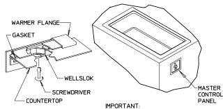
MOUNT APPLIANCE SO THAT THE MASTER CONTROL PANEL ARE LOCATED TO THE FRONT OF THE FIXTURE.
