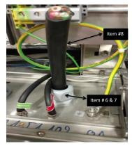
Pictured below are the incoming water lines located on the side and bottom of the oven. (The hoses shown below are included with the Convotherm 4
