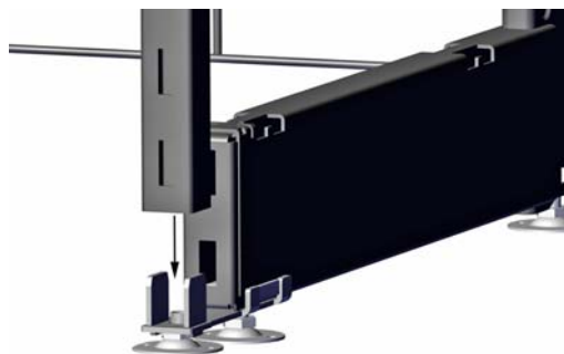
Fig. 50 Both of the front adjustable feet must be set to the same height.
