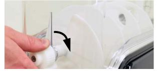
**12** Install the o-rings onto the spigot assembly. Make sure the neck of the larger gasket is facing the smaller gasket. Apply a thin film of food-safe lubricant to the o-rings.
