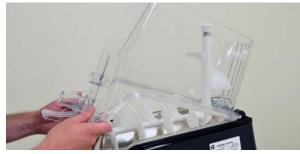
**10** Remove the gasket from the tank.
