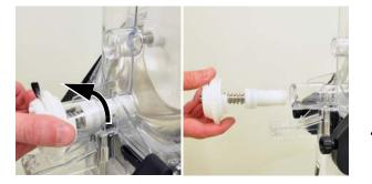
**6** Remove the o-rings from the spigot assembly and auger support knob.
