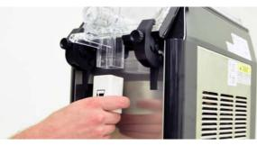
8 Remove the bowl clamp screws. Open the bowl clamps.
