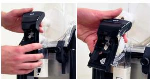
**4** Loosen and remove the auger support knob.
