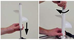
**4** Verify the bushing is in place. Press the gear onto the back of the horizontal auger.
