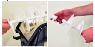
**12** Loosen and remove the nut at the top of vertical auger. Remove the auger.
