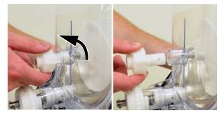
**5** Loosen and remove the spigot assembly.
