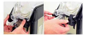
**10** Install the o-rings onto the horizontal auger support knob. Apply a thin film of food-safe lubricant.
