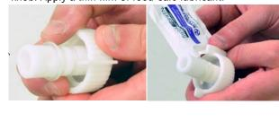
**11** Insert the horizontal auger support knob. Firmly press the knob in and turn it clock-wise.
