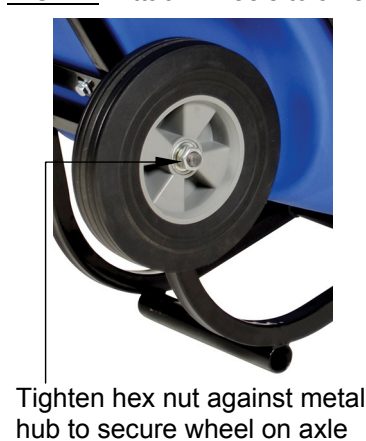
FIG. 1B: Attach wheels to axle
