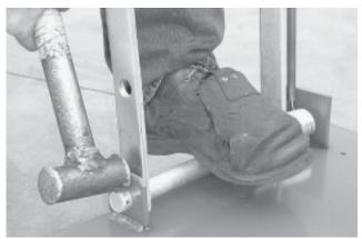
Use the hammer to push the end of the bracket back to an upright / straight position.
