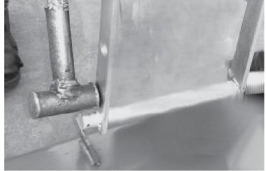
Use a hammer to "push" the release lever assembly towards the angle bracket while lifting the locking finger.
