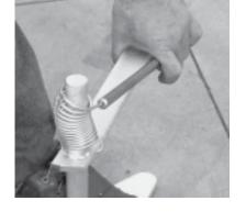
One of the easiest ways to tighten the spring tension is to put the release lever assembly on the ground and support it with your foot (as shown in picture.) Then, using the small pipe to help increase leverage, turn the spring one complete revolution to load the spring.
