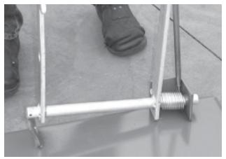
Insert the long end of the release assembly pin into the angled bracket, making sure the free end of the spring (the end with the pipe) is resting on top of the angled bracket, not on the hopper base.
