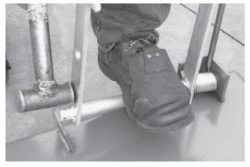
Use a hammer to push the release lever assembly towards the angled bracket while pushing down on the locking finger.
