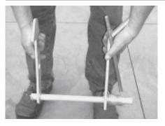
Hold the spring tube against the release handle to keep the spring from unwinding. Reinstall the release lever assembly.
