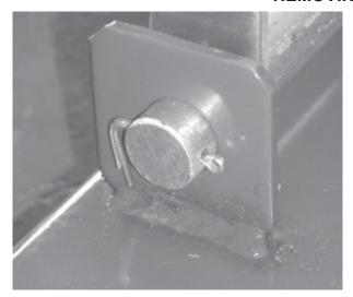
Using a pair of pliers, straighten the ends of the cotter key. Remove the cotter key.
