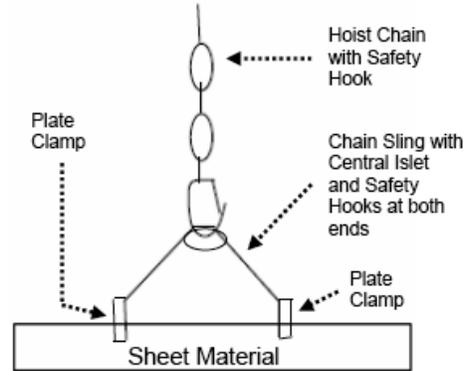
**STEP 6:** Lift the sheet to an ergonomically comfortable height. Steady the load by grasping the hoist hook or the bale of the clamp. Do not apply any weight to the top edge of the sheet material. Do not touch the lock lever. Walk slowly and move the load to the work location.
