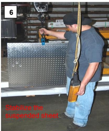
**Diagram: Using 2 Plate Clamps**
