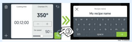
**Touch** the time or temperature space then modify the value using the key pad. **Slide** the slider to change the fan speed. **Touch** the forward arrow icon when finished.
