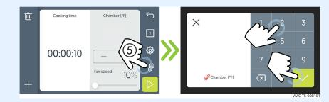
4. Now set the cooking parameters. **Touch** the cooking temperature **(6)**. **Enter** the cooking temperature using the key pad.
