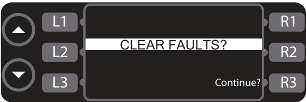
Figure 28: Confirm Clear Fault Counts Screen
