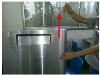
8. Take off unit cover cap from the left-top side of door, then install it in the right side of door hole.
