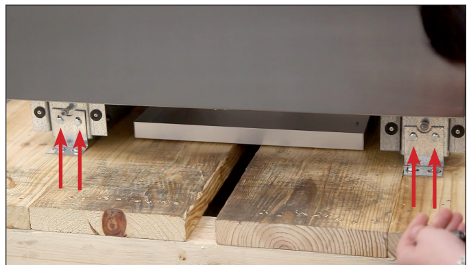
FIG. 7. Shipping bracket bolt locations.
