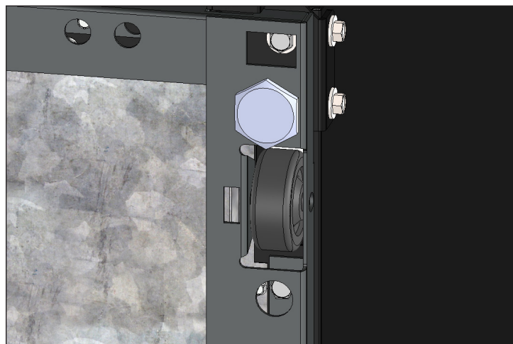
Fig. 11. Position the castor.
