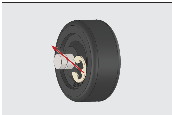
Fig. 13. Install retaining ring.
