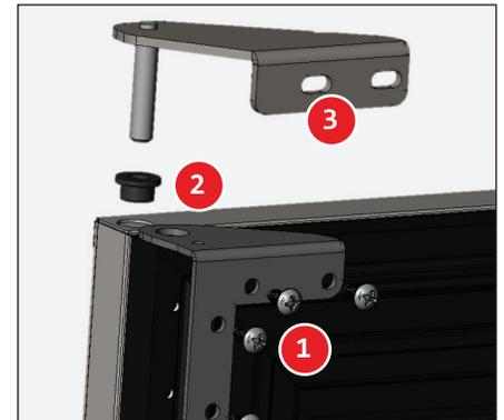
**Fig. 7b.** Top hinge component assembly.
