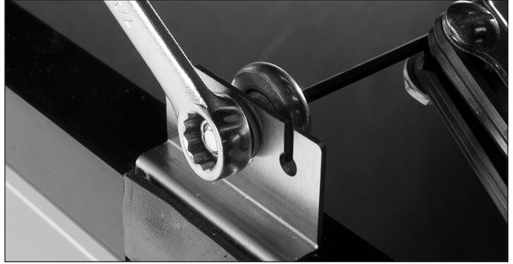
**Fig. 1.** Adjust the roller.
