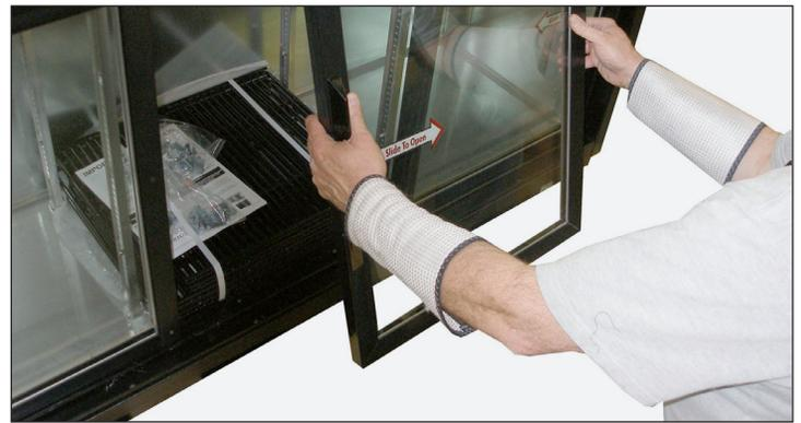
Fig. 2. Carefully remove the door.
