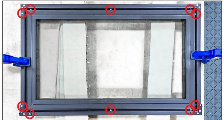
Fig. 7. Cabinet door predrilled hole locations.
