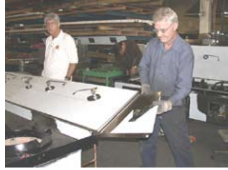
5. Sidesplash may be removed. Range will fit through 34" opening.
