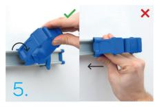
Mount the holder by hooking the top in a 45° angle. Push downwards until a click sound is heard. Error when pressure mounting.
