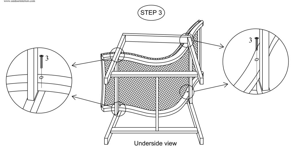
Tighten screws once the chair is fully assembled.
