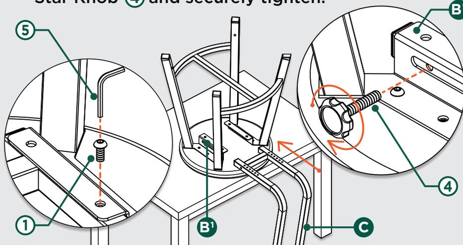
**!** Ensure that all bolts are fastened tightly.
