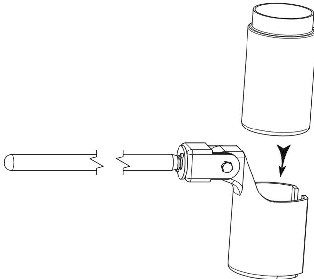
2. Adjust jar carrier to necessary angle for use with respective sampling port. Wing nut and bolt may be need to be tightened occasionally to maintain position.
