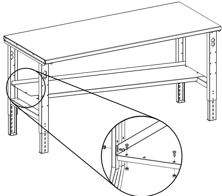
5. Attach the divider shelf to the cantilever upright frames. (See step 6 on how to attach). Using the help of an associate, place the upright frames with the divider shelf attached to the packing table. Use this as a template to mark the locations for the holes in the top. Remove the cantilever system off the top and unhook the divider shelf from the uprights.
