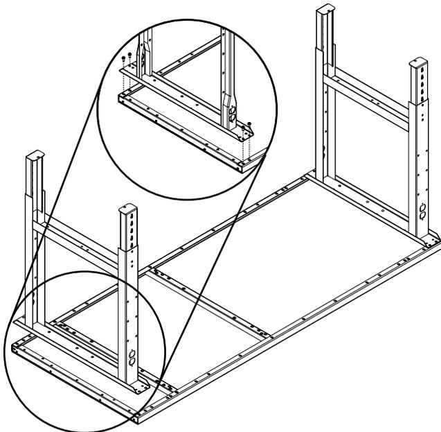
3. For assembly of a butcher block top, lay the top on a flat surface. Align the leg with the eight pre-drilled pilot holes. Attach with eight #14 x  $\frac{3}{4}$ " hex head slotted wood screws (Ref. No. 14). Repeat with second leg. Once finished, proceed to step 4.
