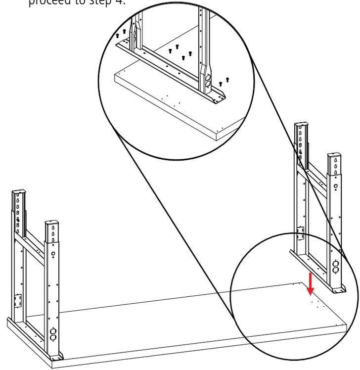
4. Turn workbench over. Place the lower shelf (Ref. No. 3) on the brace of each leg. Attach with three  $\frac{1}{4}$ "-20 x  $\frac{5}{8}$ " bolts and nuts on each end of the shelf.
