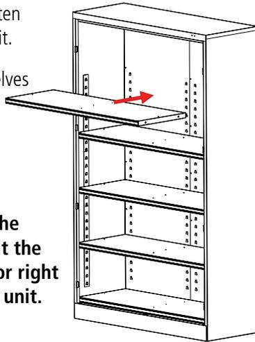
**NOTE:** In order to place the shelves, you must first tilt the shelf slightly to the left or right before inserting into the unit.
