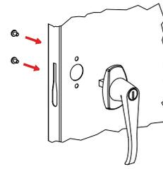
1. Place the locking handle (Ref. No. 10) on the right hand door and fasten with two #8-32 X 1/4 hex-head bolts and lock washers, provided with the handle.
