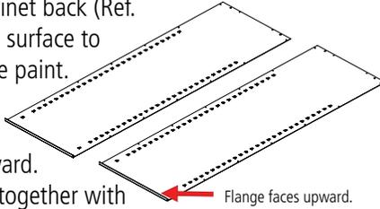
Bolt the back panels together with seven bolts and nuts (Ref Nos. 17 & 18).
