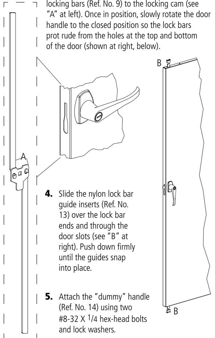
4. Slide the nylon lock bar guide inserts (Ref. No. 13) over the lock bar ends and through the door slots (see "B" at right). Push down firmly until the guides snap into place.
