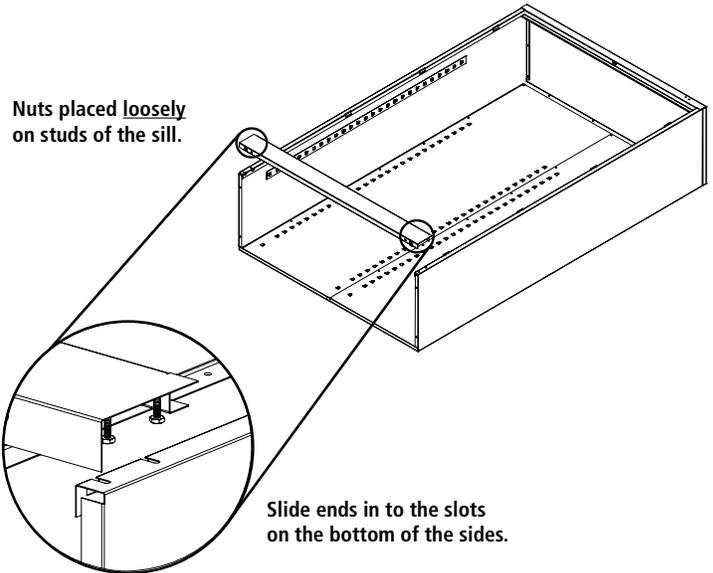
7. Place the rear flange of one of the shelves (Ref. No. 4) into the four bottom lances of the back. The front of the shelf will rest on the sill.
