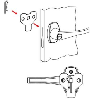
3. With the handle still in the open position, hook the locking bars (Ref. No. 9) to the locking cam (see "A" at left). Once in position, slowly rotate the door handle to the closed position so the lock bars protrude from the holes at the top and bottom of the door (shown at right, below).
