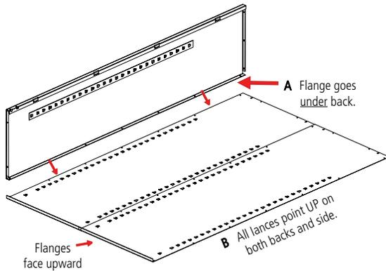
4. Attach the top (Ref. No. 5) to the unit by sliding the outer flange over the back of the unit and the side flange on the top over the side panel. The threaded studs should go through the holes in the top flange of the side and fasten with three nuts. Attach the back to the top using four bolts and nuts.
