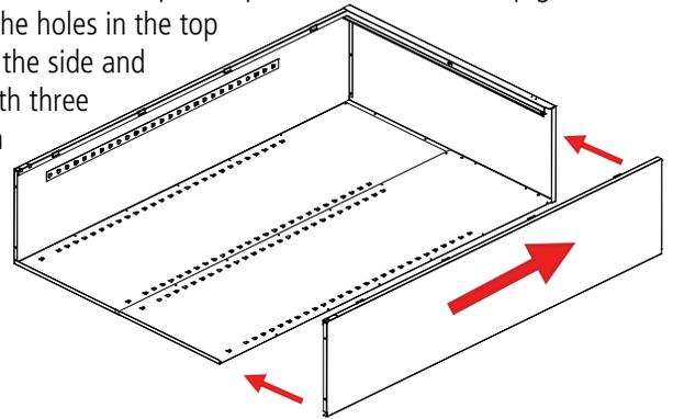
6. Attach the sill (Ref. No. 8) to the sides. Place nuts loosely on each of the studs and slide the ends of the sill into the slots on both sides of the unit. Then, securely tighten the nuts.
