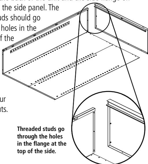
5. Attach the right side (Ref. No. 3) to the back in the same manner as you did in step 3, again, making sure that the flange is around the back and that the lances on the shelf adjustment strips are pointed in the same direction as those on the back and left side. Push the side panel up so the studs in the top go through the holes in the top flange of the side and fasten with three nuts as in step 4).
