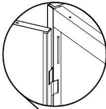
10. Attach the left door (Ref. No. 6) to the unit by placing the door on the hinges, aligning the hinge holes, and dropping the hinge pins (Ref. No. 15) into the slots. Then, tap the top of each hinge pin until fully seated.
