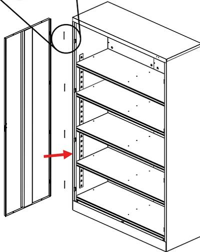
11. Attach the right door (Ref. No. 7) to the unit in the same way you attached the left door.
