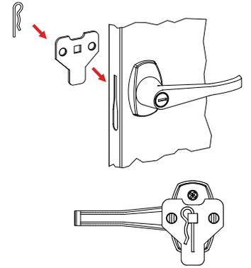
3. With the handle still in the open position, hook the locking bars (Ref. No. 10) to the locking cam (see "A" at left). Once in position, slowly rotate the door handle to the closed position so the lock bars protrude from the holes at the top and bottom of the door (shown at right, below).
