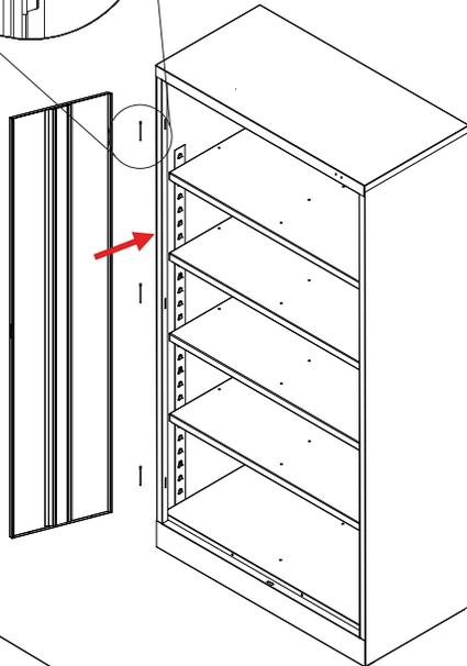
11. Attach the right door (Ref. No. 9) to the unit in the same way you attached the left door.
