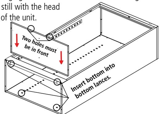
8. Set the unit upright and tighten all nuts around the entire unit.
