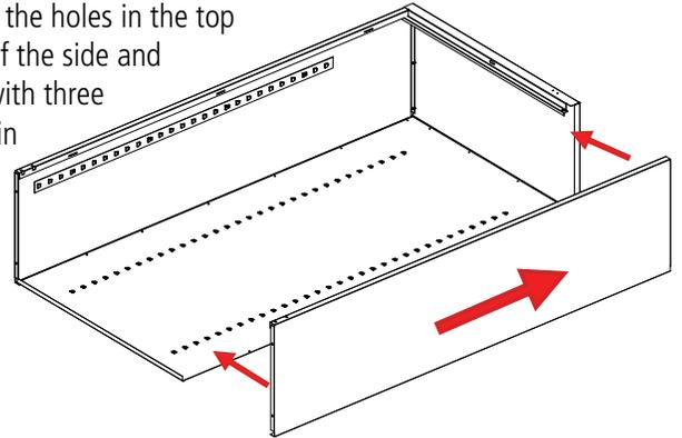
6. Attach the sill (Ref. No. 6) to the sides. Place nuts loosely on each of the studs and slide the ends of the sill into the slots on both sides of the unit. Then, securely tighten the nuts.
