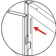
10. Attach the left door (Ref. No. 8) to the unit by placing the door on the hinges, aligning the hinge holes, and dropping the hinge pins (Ref. No. 15) into the slots. Then, tap the top of each hinge pin until fully seated.
