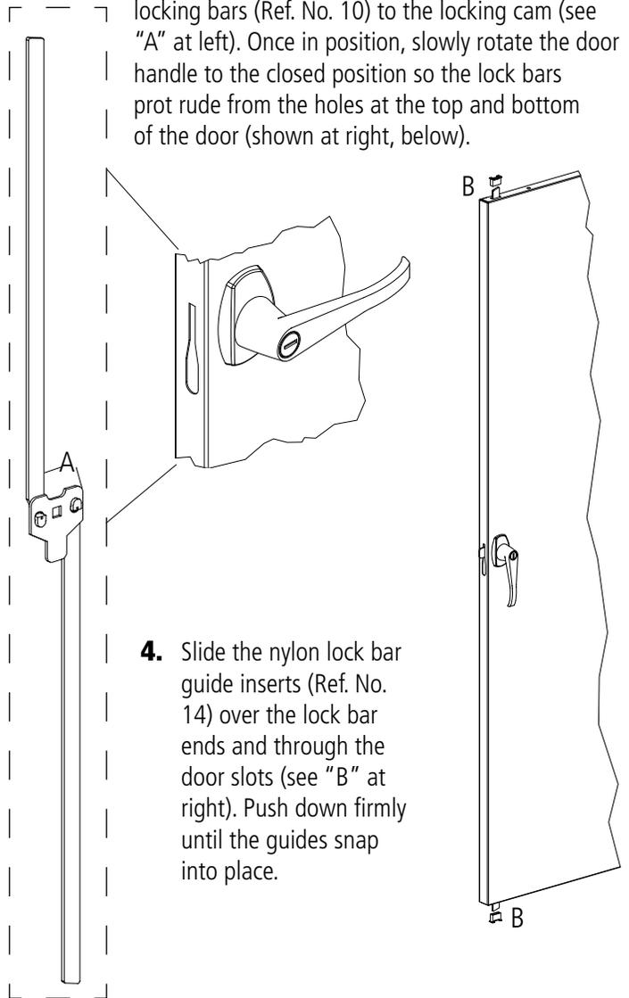
4. Slide the nylon lock bar guide inserts (Ref. No. 14) over the lock bar ends and through the door slots (see "B" at right). Push down firmly until the guides snap into place.
