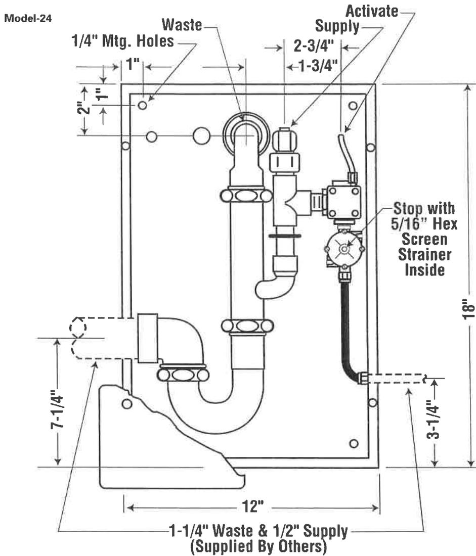
**NOTE:** Frost-proof cabinet has pre-manufactured holes, so unit can be plumbed from either right side (shown) Or left side.
