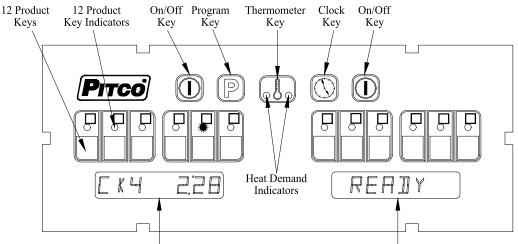
Displays show current operation. Throughout this text, a left only display will be printed as [CK4 2:28]. When both left and right displays should be interpreted together, this text will show them as [CK4 2:28] [READY ].
