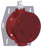
Carefully install the new Red Pump Assembly onto the six(6) 1/4-20 studs in the Handle Assembly. Very loosely install the six(6) 1/4-20 flange nuts onto the studs.
