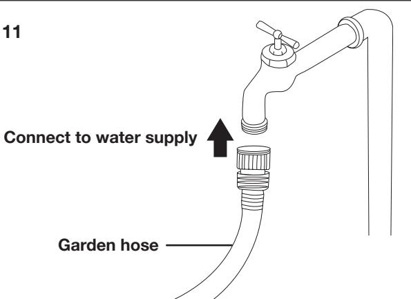
**⚠️WARNING!** Do not connect to potable water system.
