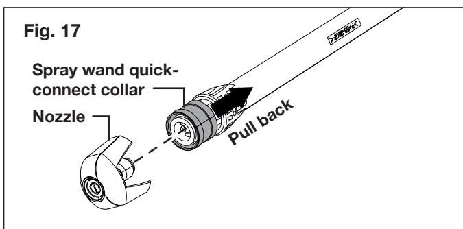
To disconnect a nozzle from the spray wand once the cleaning job is complete:
