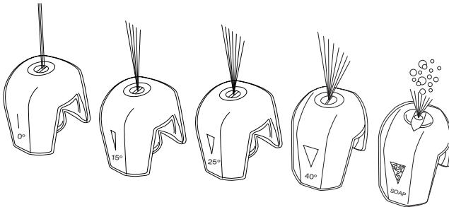
I) The 0° intense-jet nozzle (red) is an extremely powerful nozzle that delivers a high-pressure, pencil-point jet stream. It is used to cut heavy dirt deposits in a small, concentrated area. It is ideal for dissolving stubborn substances, like tar and grease spots on concrete, or for removing caked mud from equipment. Use this nozzle to clean hard-to-reach areas including the facades of 2-story buildings or the undersides of lawn mowers and tractors.
