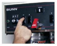
10. Place an empty server under the 11. Place "ON/OFF" switch in lighted upper position.
