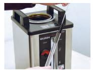
10. Unscrew the sight gauge cap. 11. Clean the sight gauge with the large brush (00675.0000) and reassemble.
