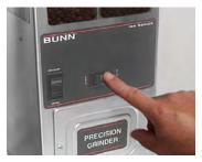
For two hopper grinders, select coffee type by pressing "RIGHT" or "LEFT" hopper. Skip this step for 1 hopper grinders.
