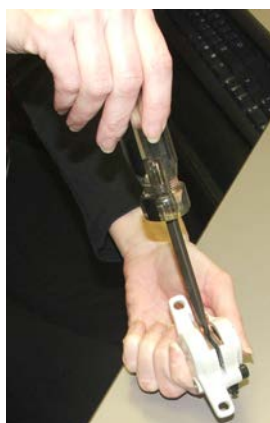
Figure 2 Compressing the piston
