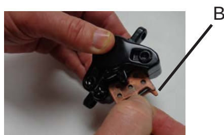
Figure 5 Inserting the pads
