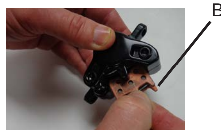
Figure 3 Removing/Inserting the pads
