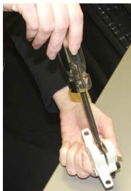
Figure 2 Compressing the piston
