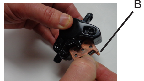
Figure 3 Removing/Inserting the pads
