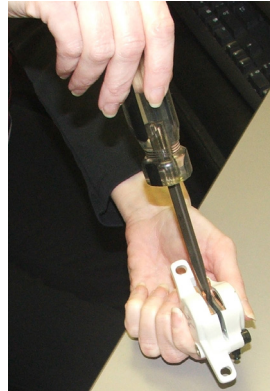
Figure 2 Compressing the piston
