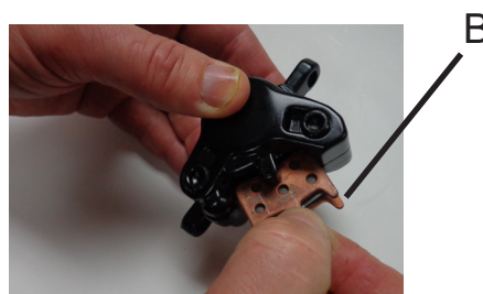
Figure 5 Inserting the pads
