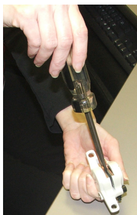
Figure 2 Compressing the piston
