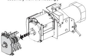
**D.** Now the blade assembly will be free from the housing. Completely remove the blade assembly from unit.
