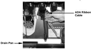
Locate the ADA harness, units with a crusher it will be on the left of the ice chute, non-crusher units will be on the right. Continue routing the ADA cable behind the valve mount cap up towards the ADA harness.
