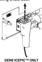
Remove the decorative ice chute by pulling the cotter pin out on the right side of the chute rod and pulling the chute rod toward the left side of the dispenser.
