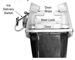
Begin by observing the chute while slowly pushing against the rocking chute. When the ice delivery switch clicks, measure the distance from the door stops on the rocking chute bracket to the door. The distance between the two must be no more than 1/4" (0.64 cm), but no less than 1/16" (0.16 cm).
