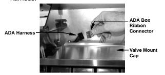
6. Connect the ADA ribbon cable to the ADA wire harness that is fastened to the foam front by a wire clip.
