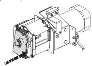
5. Replace the crusher drip pan, sliding it until it snaps into place by pulling up slightly on the crusher assembly and pushing the drip pan toward the foam front.
