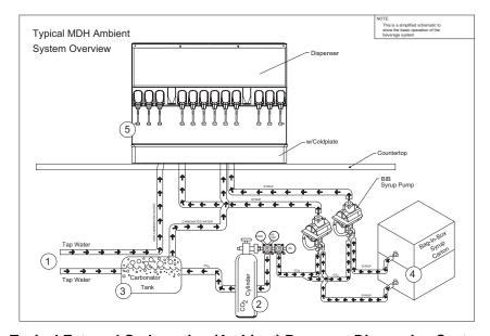
Typical External Carbonation (Ambient) Beverage Dispensing System
