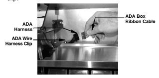
7. Neatly tuck in and take up any slack remaining in the ADA ribbon cable so it will not be in the way of any moving parts or panels when they are placed back on the unit.
