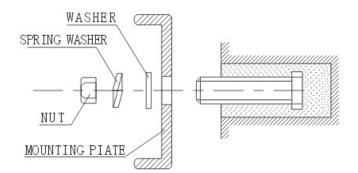
Drill anchor points in the wall and fix the bolts in the proper position. Use the mounting plate as a template to mark the fastener locations.
