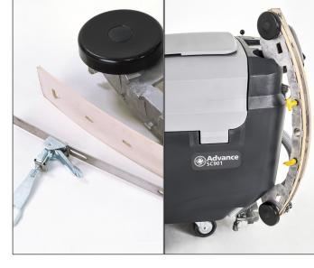
15. Clean and inspect the squeegee blades. Flip the blade or replace it if required. Hang the squeegee on the machine as shown. Tan Gum Rubber Blades – pn 56115334 Red Linatex Blades – pn 56115333
