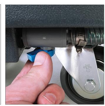
2. Check the solution shut off valve.
