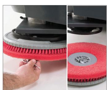
14. When finished using the machine, remove the pads or brushes. Inspect and clean or replace them as required.
