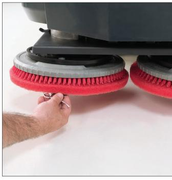
2. Inspect the pads/brushes for wear and replace as required. 14 in Pad Driver – pn 56505800
