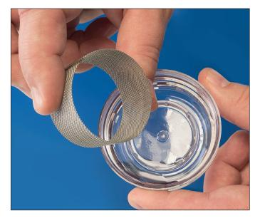
4. Inspect and clean the solution filter as required. Filter – pn 56104351.
