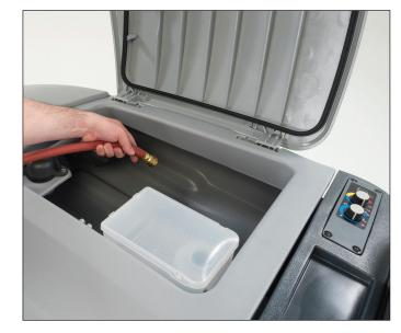
16. Rinse the recovery tank and leave the lid 17. Inspect the float ball cage. open to dry.
