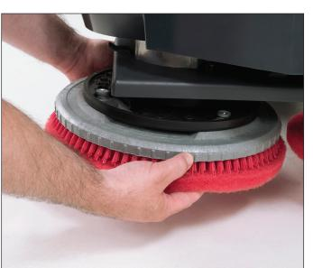
1. Turn the machine on and check the status 2. Inspect the pads or brushes for wear and install them on the machine. Lift the lugs into the slots and rotate the brushes to lock them into place.
