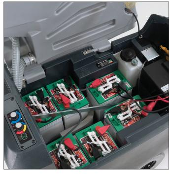
1. Check the level of the batteries and add distilled water as required.
