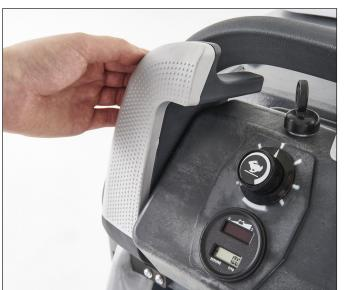
6. Press the paddle forward to transport the 7. Pull the paddle backward to go in reverse. 8. Lower the scrub deck to the floor using
