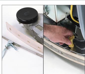
3. Check the squeegee blades for wear and flip or replace if worn, nicked or torn. Install squeegee and hand tighten thumb nuts.
