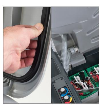
2. Inspect the recovery tank gasket and hoses.
