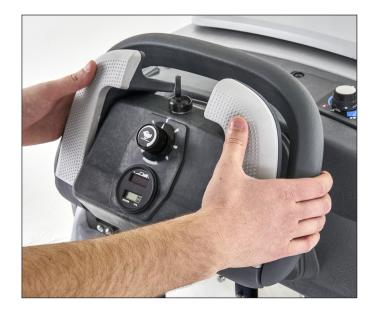
11. Propel the machine forward using the paddle.
