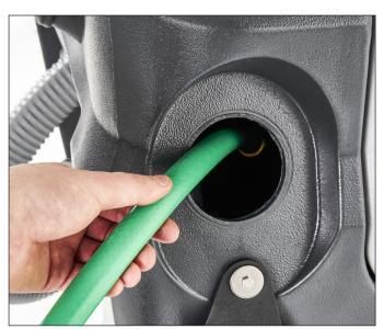
5. Fill the tank with the appropriate cleaning solution. Black Cap – pn 56115395
