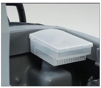
13. Inspect and clean the debris catch cage. Refill the clean water tank as required.
