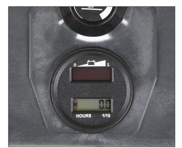
of the batteries. If two bars or less are showing, charge the machine for 2 to 8 hours.
