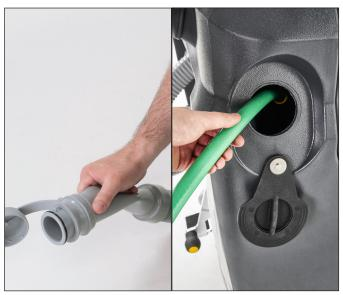
12. When the vacuum motor changes pitch the recovery tank is full and needs to be emptied. Refill the clean water tank as required.
