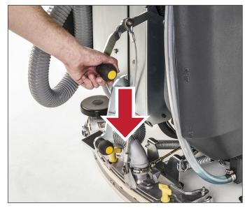
9. Lower the squeegee to the floor and the 10. Select the desired solution flow rate vacuum motor will start.
