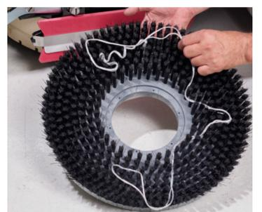
15. Turn the brushes counter clockwise and remove the brushes or pad holders. Rinse the brushes or pads in warm water and hang up to dry.
