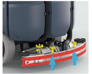
5. Check the squeegee blades are not damaged and install the squeegee by turning the yellow knobs. Check the height of the squeegee by adjusting the castor wheels and the angle knob.
