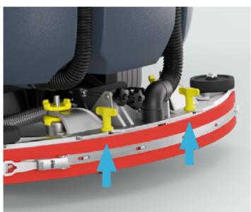
16. Untighten the yellow knobs, take the squeegee off and remove debris. Check and clean the squeegee blades.
