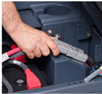
3. Check battery cables are well connected together.
