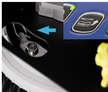
8. Lift the brush and rotate to the left to lock into position. If click-on option is available, align brush directly below motor using alignment system and push brush install button. (Disc version only).
