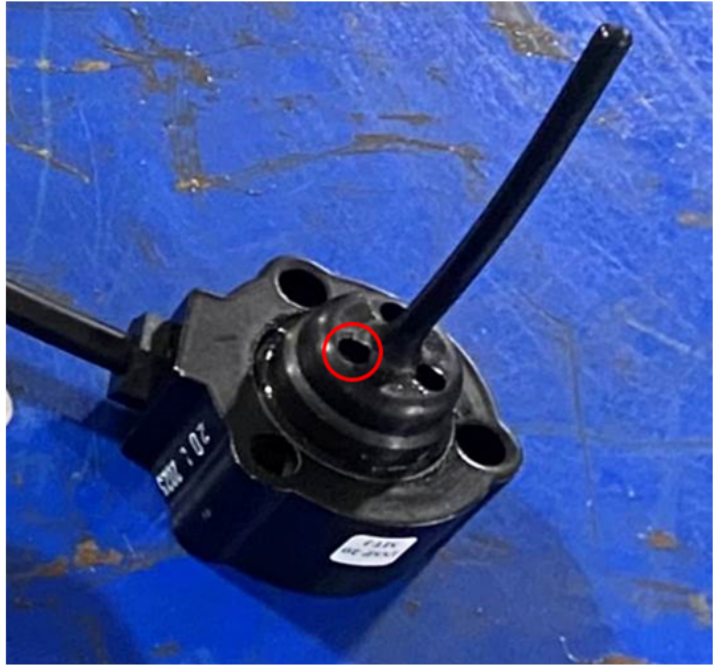
New Probe- 3 holes filled with epoxy/resin
