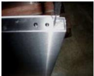
10) Install the original cartridge into bottom left corner where you just removed the foam from and install the black screws onto this side of the door
