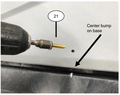
Install Screws #13860 in remaining 4 holes in panel into base using of 3/8" Nut Driver bit. Repeat sequence to assemble other side panel to base. Install (5) Screws #13860 in 5 holes in rear panel into base using of 3/8" Nut Driver bit.
