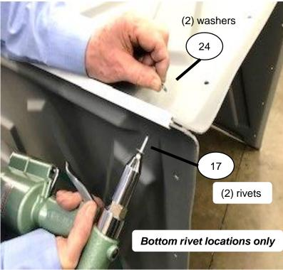
**Step 4: Assemble 3 Panels to Front:** Pull 3 assembled side panels onto base & front assembly. Install corner molding # #22989 between the panels & front (notched end of corner molding at top of panels). Fasten panels, start in middle of panels use (16) Rivets #11030 and (16) Washers #11315 (rivet from side panel). Bottom hole on panels use longer rivet, (2) Rivets #22543 & (2) Washers #11315. Repeat sequence to assemble other side panel to front panel.
