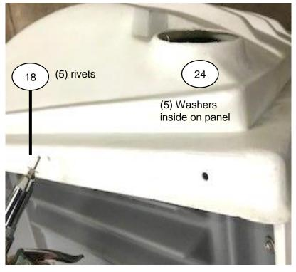
**Step 9: Assemble Roof to panels & front (continued):** Drill through 5 holes in roof (5 dimples if roof has no holes & panel has no holes) through side panel using #10 Drill Bit. Fasten roof to side panel using (5) Rivets #11030 outside on roof & (5) Washers #11315 inside on panel. Repeat sequence to assemble roof to other side panel.
