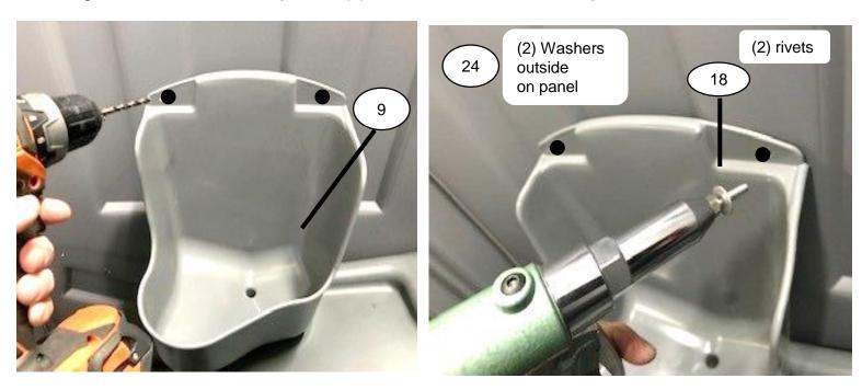
**Step 8: Assemble Paperguard hood to panel:** Drill out 2 dimples in top recess tabs in PaperGuard hood #22917 using #10 Drill Bit. Drill out 2 dimples in right panel using #10 Drill Bit.
