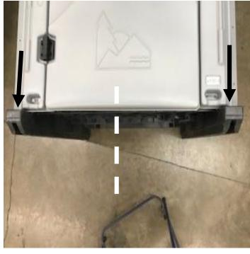
Install (4) Screws #13860 in holes on left & right side of front (door frame) at bottom, using a 3/8" Nut Driver bit (DO NOT over tighten screws, run screws in until rubber washer begins to flatten).
