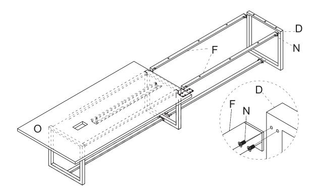
Use the Screw (M) to connect the Frame and the Top (O), Use the Screw (N) to install the Bracket (J) to the Top;
