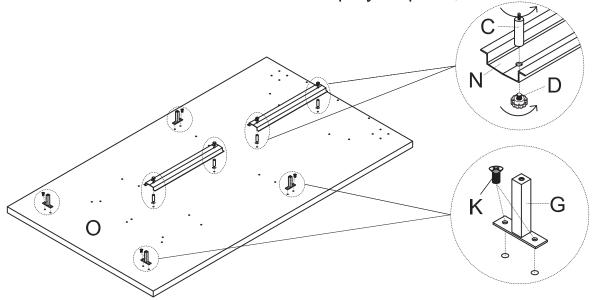
Use the Screw to connect the Legs and the Frame (A) to the Top (O). Use the Screw (K) to connect the Metal Plate (E) with the Top (O);
