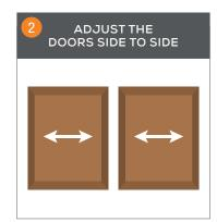
Slightly turn the adjusting screw (D) on both hinges on each door. You may have to slightly release the locking screw C to do this. Make sure it's tight afterwards
