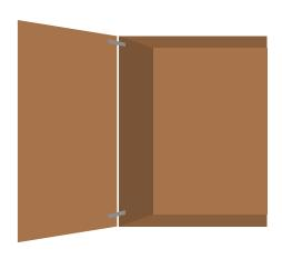
If the door is not closing properly or is making creaking sounds it may be binding on the cupboard frame.
