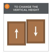
Undo the two adjustable cupboard screws (B) on both hinges. They are usually in slotted holes, which means you can adjust up or down by a few mm, then tighten back up.
