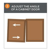
Use the adjusting screw (D) but this time only screw either the top or bottom screw. For a bigger adjustment, screw the top one way and the bottom the other! You may need to slightly release the locking screw (C) to do this. Make sure it's tight afterwards.
